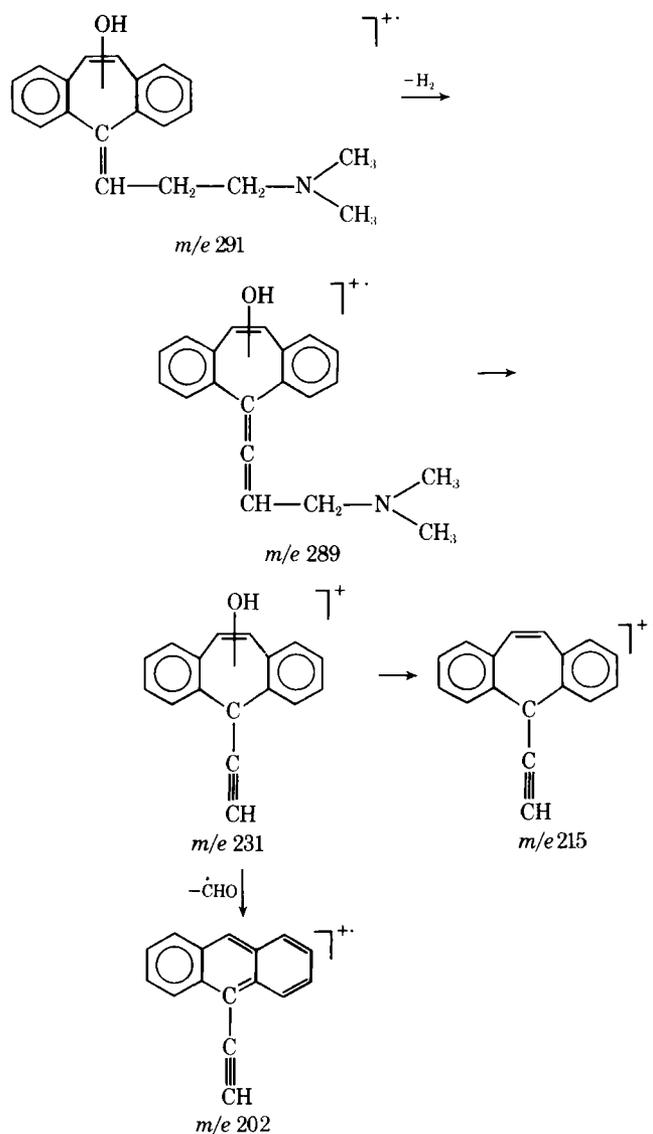
Scheme III—Suggested fragmentation pathway of hydroxycyclobenzaprine. (No exact mass measurements were included in the parent ions or fragments, and only a few metastable ions were available to support the fragmentation scheme.)
