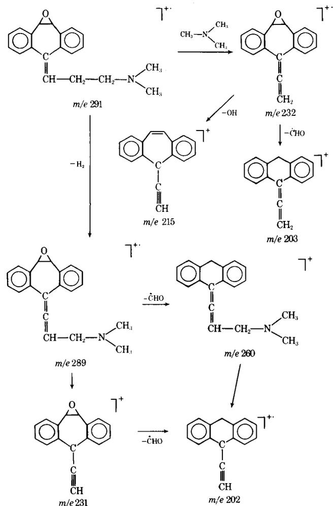
Scheme II—Suggested fragmentation pathway of the 10,11-epoxide of cyclobenzaprine. (No exact mass measurements were included in the parent ions or fragments, and only a few metastable ions were available to support the fragmentation scheme.)
